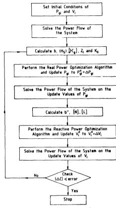
Figure (2): Iterative Procedure
