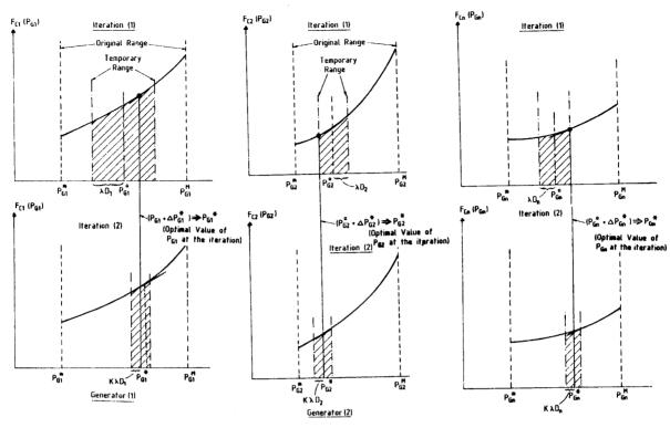
Figure (1) Graphic depiction of the Section reduction Method.
